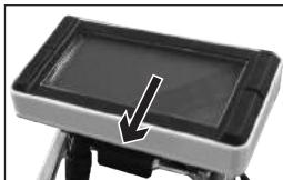
**NOTICE.** To prevent loss of riding information, please make sure that the controller is switched Off before it is removed from the bike.
